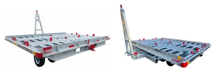
Suitable for loading and unloading P1,P6,P7,P9 pallets and LD1, LD2,LD3,LD4,LD6,LD7 containers.
