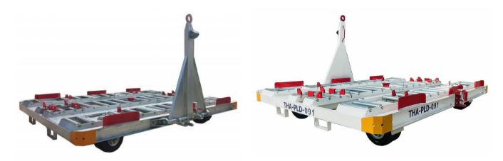
Suitable for loading and unloading P1,P6,P7,P9 pallets and LD1, LD2,LD3,LD4,LD6,LD7 containers.
