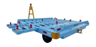
Suitable for loading and unloading P1,P6,P7,P9 pallets and LD1, LD2,LD3,LD4,LD6,LD7 containers.
