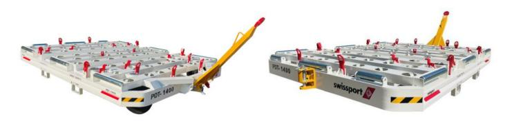
Suitable for loading and unloading P1,P6,P7,P9 pallets and LD1, LD2,LD3,LD4,LD6,LD7 containers.
